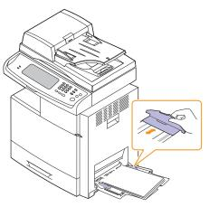
**5** After loading paper, set the paper type and size for the multipurpose tray. See page 4.9 for copying and faxing or the **Software section** for PC-printing.
